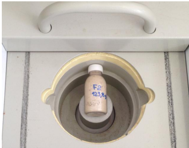
Fig. 4. Location of the flask on the detector of gamma-ray spectrometer.
